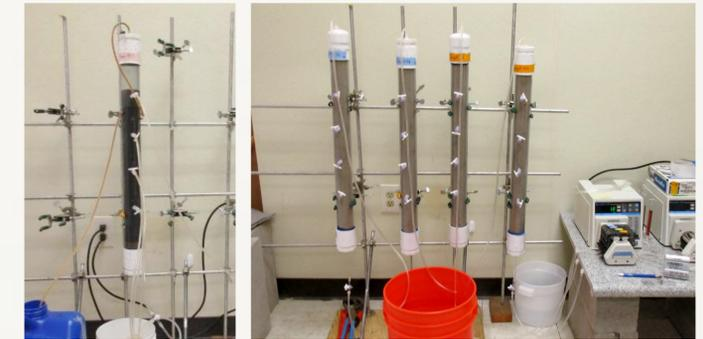
Figure a. Multiport Columns: Left: ZVI Only; Right: ZVI+Sand
